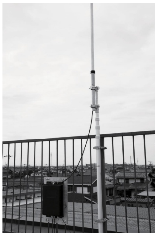
(Picture-2) Installing the ATU far from the mast. ATU is the CG3000.
