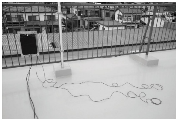
(Picture-3) 2pcs 5m(16.4ft) ground wire (counter poise).
